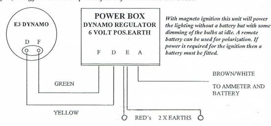
MOUNT IN ANY POSITION, THE LUCAS COVER CAN BE PUSHED OVER THE UNIT AND HELD WITH LOCKING WIRE OR CLEAR PLASTIC STRAP. THIS WILL GIVE AN ORIGINAL APPEARANCE WHEN REQUIRED
