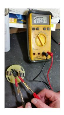
Note the reading for the Dt1a & SS4 plate will be around 65 ohms for both tests as these are single coil plates.
